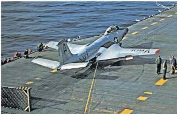
An early F2H-3 assigned to VF-141 is ready to launch from Cat 2 aboard USS RANDOLPH, CVN-15, in 1954. The oldest shades of metal are evident on the natural metal surface. Magnesium panels, non-cold aluminum panels, and fiberglass surfaces were painted with aluminum lacquer. (NAMM)
