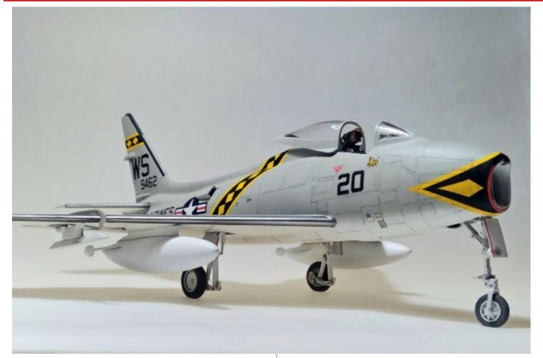
The FJ-4B had a strengthened wing with three hard points per wing instead of two on the FJ-4 and the Low Altitude Bombing System (LABS) for delivering tactical nukes. The FJ-4B also had a second set of speed brakes added low on the fuselage near the tail pipe. The second set of speed brakes is the visible difference between the FJ-4 and the FJ-4B.
