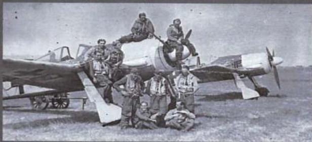
Two white-cowled Fw 190 A-4s seen in Deelen during April/May 1943, most probably belonging to 1/JG 1 following the re-designation of IV. Gruppe (on the establishment of JG 1). The purpose of the overall white engine cowl was to aid unit reformation in the air after the first pass through the bomber boxes. Note the mottled speckled finish of 76 Heilmäul 'dots' over the fuselage greys on the aircraft nearest the camera. Visible under the wing of the second Fw 190 is the antenna mast for the FUG 16 ZE.
