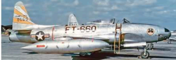
The short range of the Shooting Star in Korea led to a modification of the Fletcher tank to increase the amount of fuel that could be carried. In most cases, two extra center sections were added to the tank, as seen on this F-80C assigned to the 80 th Fighter Bomber Squadron. With these tanks, the total fuel capacity was increased by 220 gallons (110 gallons in each tank), thus significantly extending the range and loiter time of the aircraft. This modification had been evaluated unofficially in 1949, prior to the war, but it had never been approved. Once the war in Korea began, and with the F-80s having to operate from Japan in most of the early months, General Earle Partridge, the commanding general of the Fifth Air Force, authorized the use of these tanks. They became known as the Misawa tanks, because they allowed F-80Cs to operate more effectively from Misawa and other bases in Japan. However, care had to be taken while pulling "G" forces during maneuvers with the much heavier tanks when significant amounts of fuel remained in them. (G. Balzer Collection)
