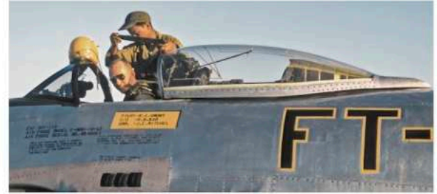
The new electrically-operated canopy was retrofitted to F-80Bs and early F-80Cs that had the original manually-operated canopy, and it became the production standard for late production F-80Cs. This canopy did have the sense antenna embedded into it. This version of the later canopy is shown here on an F-80C-10-L.O. (G. Balzer Collection)
