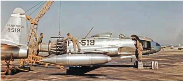
The 49 th Fighter Group insignia is just visible on the open gun bay door of this F-80C as it undergoes an engine change at Taegu Air Base in 1951. The blue marking on the nose indicates assignment to the 7 th Fighter Bomber Squadron. Another airman stands on one of the ammunition boxes as he checks out the radio gear at the aft end of the nose compartment. (Bell Collection)
