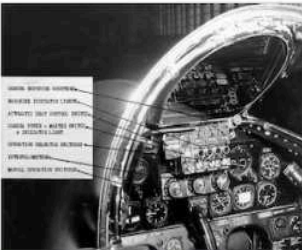
The gun sight was removed from RF-80As, and it was replaced with the control and indicator panel for the camera equipment. The installation of this panel also necessitated the rearrangement of some of the instruments and gauges. (NMUSAF)
