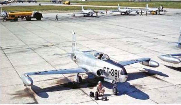
The first jet powered tactical reconnaissance aircraft to enter service with the U. S. Air Force was the RF-80A. This was a rather simple and straight-forward modification that replaced the standard nose and its six .50 caliber machine guns with a longer and larger nose to house cameras and their associated equipment instead. A pilot assigned to the 160 th Tactical Reconnaissance Squadron of the 117 th Tactical Reconnaissance Wing at Neuburg Air Base, Germany, poses with a K-17 aerial camera in front of an RF-80A in May 1952. (Bell Collection)
