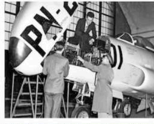
P-80A-1-LO, S/N 44-85201, was converted to serve as the prototype for the photo reconnaissance version of the Shooting Star. After the lengthened and modified nose was installed, USAAF representative, LtCol. Matos, inspected the prototype which was initially designated the XFP-80A. (NMUSAF)
