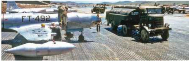
The second type of fuel tank to be carried under the wing tips was manufactured by Fletcher. It had a much more pointed nose than the original tanks, and it was made in three sections with the center section being cylindrical in shape. One is seen here under the right wing tip of Baird Martin's (to whom this book is dedicated) F-80C in Korea as the Shooting Star is being refueled. Note the open filler cap on the tank. (G. Balzer Collection)
