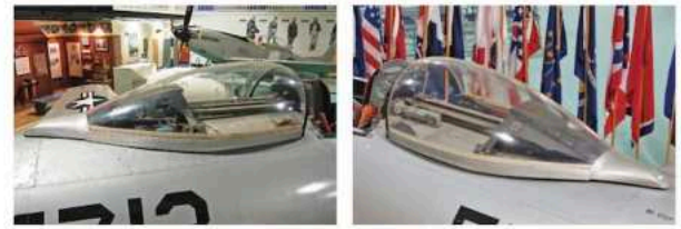
The canopy on the F-80C that is displayed at the U. S. Air Force Armament Museum is simply placed on top of the fuselage aft of the cockpit, and it is not connected to its rails inside the cockpit. This places the canopy farther aft on top of the fuselage than it would be on an operational aircraft. However, these two photographs are included to show the details of the rails aft of the seat that were part of the mechanism on which the canopy moved fore and aft as well as the structure inside the aft end of the canopy. The small yellow item seen in the photo at left is the manual canopy release. (Both, Kinzey)
