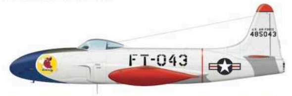
F-80A-1-LO, S/N 44-85043, was assigned to the 33 rd Fighter Squadron of the 4 th Fighter Group in 1948. By this time, the designation had been changed from P-80A to F-80A. The pilot probe had been deleted from the leading edge of the vertical tail, and a small L-shaped probe had been added under the nose. Note that this aircraft was painted in silver lacquer, rather than being natural metal. (Roszak)
