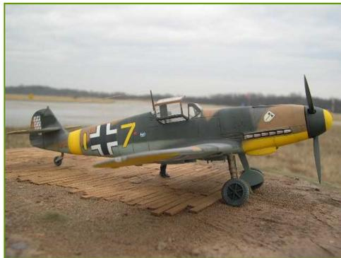
add it you can. I will add mine later if I want it. I used *Solvaset* and the decals performed flawlessly. I wish they all worked as well. Sealing the decals with another gloss coat and then a coat of flat it was time for a little weathering.
