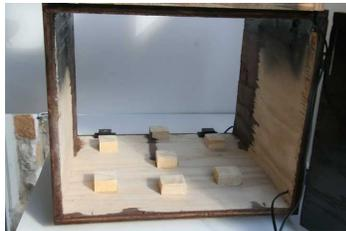
I took the drawing with me so the person who used the saw could see what I needed. Once I had all the pieces, I assembled the outside box by gluing, drilling pilot holes and nailing it together.
