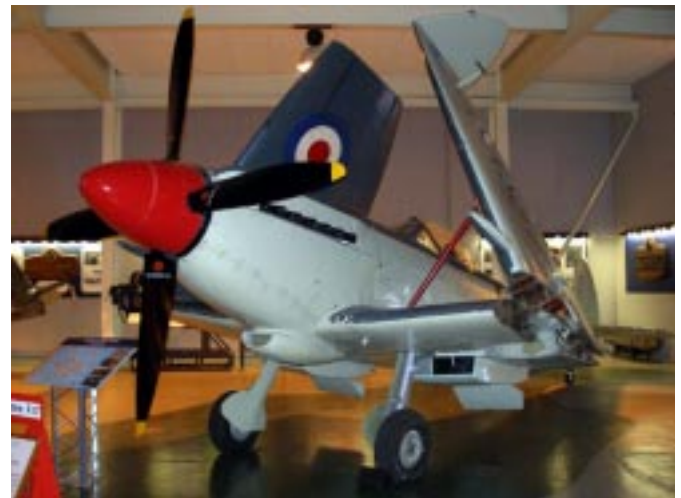
Griffon powered Supermarine Seafire F.17. Earlier mark Seafires delivered to FAA did not have wing folding capability.
