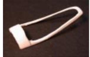
Accordingly, I poured an additional canopy shape and cut away much of the resin to leave only a frame, which, of course, nests perfectly within the vac outer shell. The finished canopy mounts to the fuselage spine via a brass pin.
