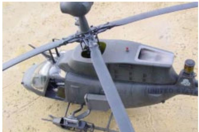
**Step 8-**One of the best things about this kit is the rotor system. It is *EXACTLY* the same as the real thing. Care and test fitting will be rewarded with an excellent representation of the real thing. A few words of caution though. Caution 1-The Pitch Change (PC) links are offset 45 degrees from the pitch horn. This is not pointed out very well. Caution 2-The blades are the
