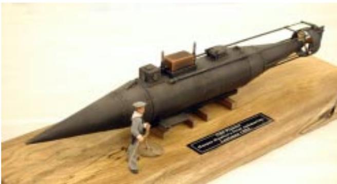
Although no detailed plans survive, this representation is based on the sketch and description submitted to the Union Department of the Navy when the boat was examined in 1862. She was 34 feet long, powered by three men turning a hand-operated winch and steered by a fourth man with hand operated rudder and diving planes.
