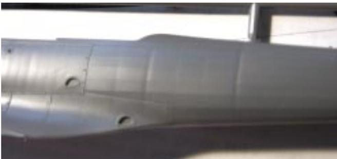
You have to fix this and it's not all that hard. What you need is a bottle of Mr. Surfacer, some cotton balls, and some alcohol. Use either isopropyl, denatured, or gin—if you're desperate. Just give the offending area two or three coats of Mr. S or whatever it takes to completely fill the sunken area and a little more. Wait until it completely sets. I recommend at least overnight. When it's hard enough to not dent easily with your fingernail, it's probably cured.
