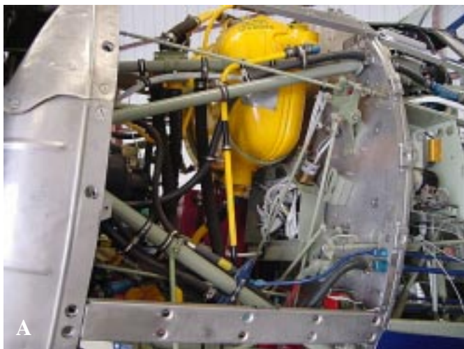
A. Oil Tank, Engine Mounts and Firewall B. Cockpit Area, left side C. Rear Instrument panel D. Left Wing and Fuselage E. Rudder Pedals
