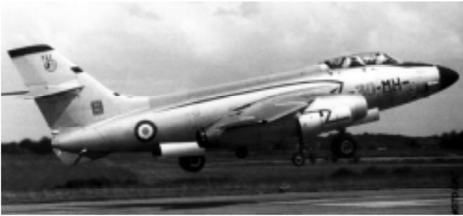
The twin-engined Sud Aviation Vautour, an esoteric-but-little-produced (approximately seventy) French aircraft of the Fifties, rose to distinction dressed in Israeli camouflage in the 1967 Six-Day War. The airframe is unusual in that its main landing gear is of bicycle configuration, as in the B-47, XB-51, B-52, Yak-25/28 and U-2. Smaller outrigger landing struts retract into the side of each engine nacelle.
